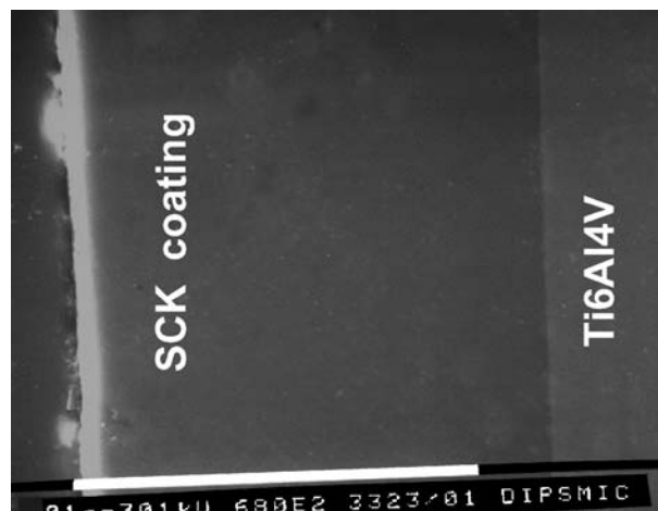
Figure 8 Cross section of a non over-reacted coating on Ti6Al4V.
